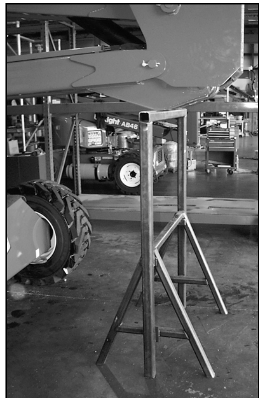
Figure 3-7: Elevating Assembly Brace
