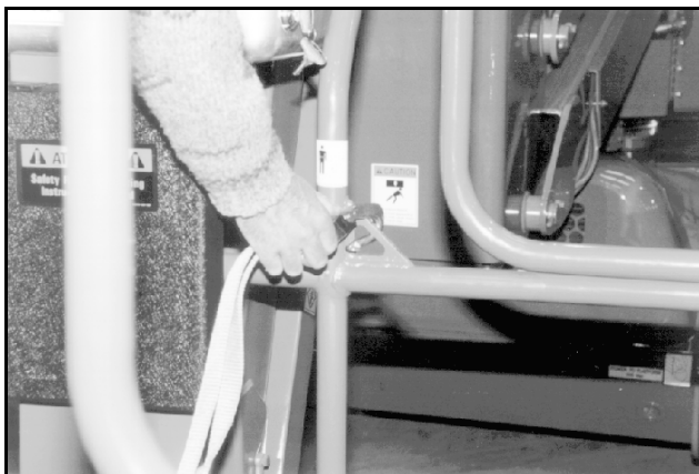
Figure 2-5: Typical Fall Restraint Anchorage Point
